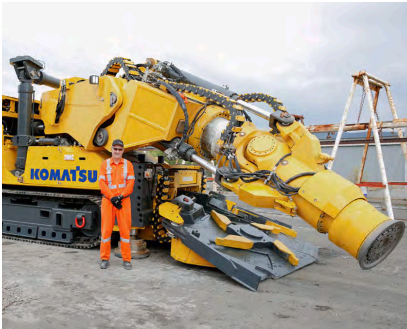
➤ Komatsu's MC51 all electric hard rock continuous miner designed and built in Australia.
