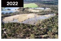
Stawell Gold Mines (SGM) is undertaking progressive rehabilitation of Davis Pit, backfilling the site using underground waste rock.
