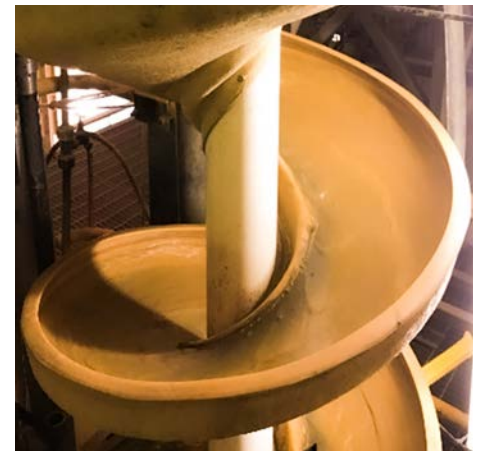
■ Processing 'spirals' are used to separate valuable heavy minerals from sand.
