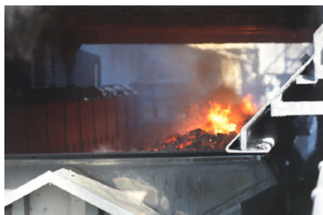
FIGURE 16: HOT COKE AFTER BEING DISCHARGED FROM A COKE OVEN
