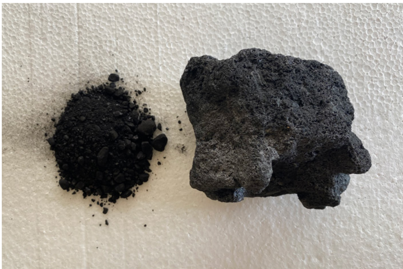
FIGURE 5: CRUSHED COKING COAL (LEFT) PRIOR TO COKING AND A LUMP OF COKE (RIGHT) AFTER COKING
