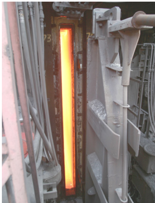
FIGURE 2: INSIDE AN EMPTY COKE OVEN AFTER COKE HAS BEEN DISCHARGED
